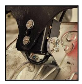
Then screw the motor securely into the holder using thread locker and 2x M5 screws.
