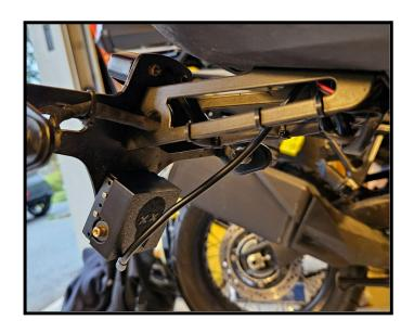
Place the control box under the seat and connect the motor to the control box (short cable).
