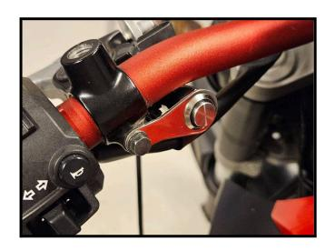
Example image with button: "Button for brake lever mount"
